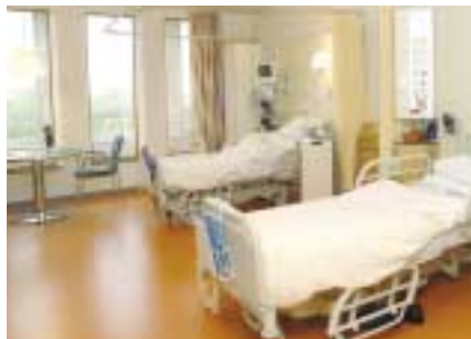
All air system without radiators near the facade allows free arrangement of rooms.
